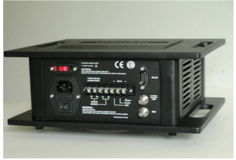
Titanium Satellite's ASC1 dish mover, polarity controller can be used as a stand-alone big-dish driver or interface with an FTA receiver. Heavy construction with many connections and easy to read display are among its attributes. (Photo courtesy of the author).
