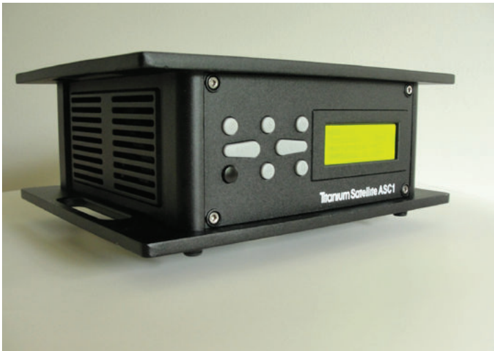
Titanium Satellite's ASC1 dish mover, polarity controller can be used as a stand-alone big-dish driver or interface with an FTA receiver. Heavy construction with many connections and easy to read display are among its attributes. (Photo courtesy of the author).
