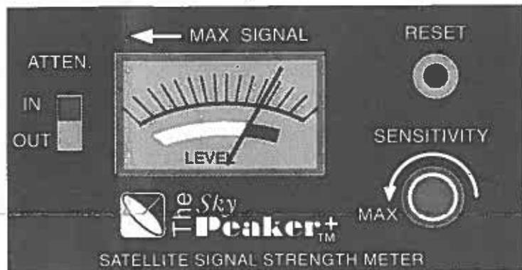
**10. CONTINUE TO AIM THE ANTENNA;** repeat steps 8 and 9 above until no further antenna movement results in a increase (toward MAX SIGNAL) in needle position.
