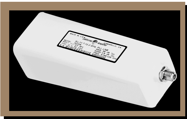
#150338/Ku-band 11.7-12.2 GHz input, 950-1450 MHz Output, Noise: 0.8dB, \pm 25 kHz
