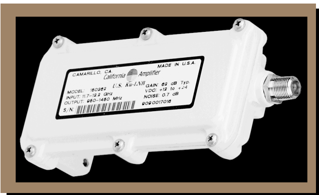
#150297/High Stability Ku-band, 11.7-12.2 GHz Input, 960-1450 MHz Output, Noise: 0.8dB
