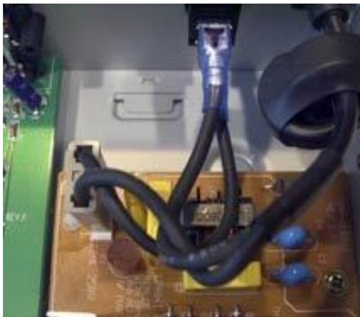
I like to reconnect things the same way they were originally connected so I used a felt tip pen to mark a letter “T” on the top wire connection to the switch. (Left picture) The power plug already had a white dot on one side so I made a mental note of it. (Right picture)
