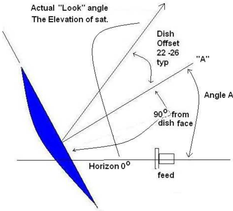
Notice that the actual angle above the horizon to the sat is Offset from the elevation of the face of the dish. If you don't know the offset of your dish, it can be calculated after making a few measurements.
