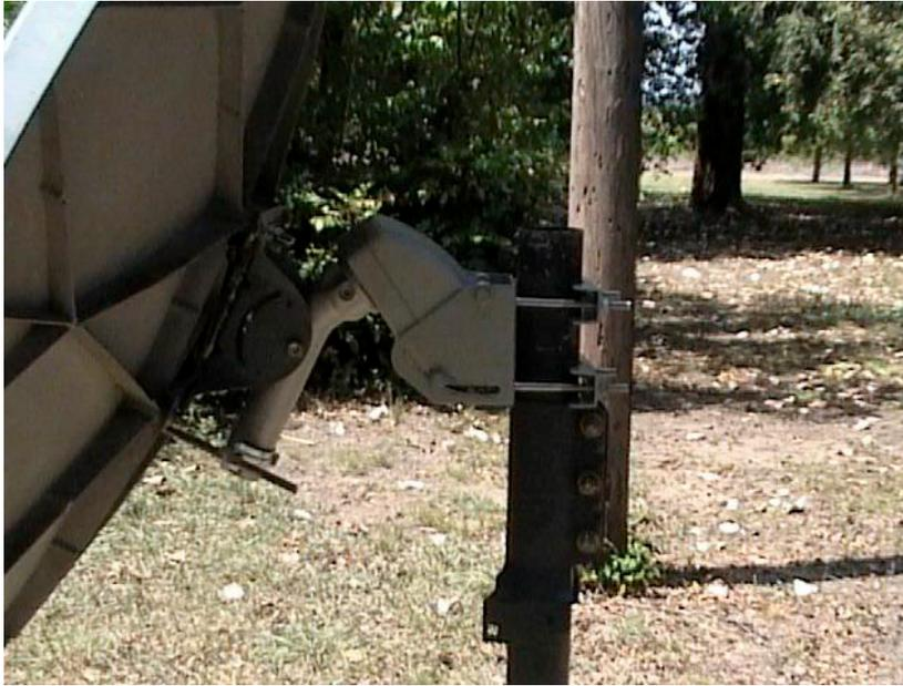
This is my setup of the Primestar 1.2 meter on the SG2100 motor.
