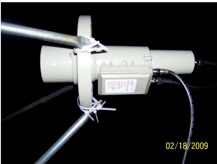
You can easily install these Ku LNBFs on Primestar 1 and 1.2 meter dish:
