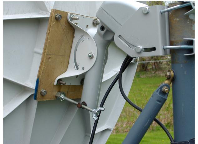
Old Primestar dish upside down on motor mount for FTA reception. Actually the dish is right side up, but the mount is upside down to make it work with the motor. You can see some PVC used as a shim to make the mount fit the motor shaft.
