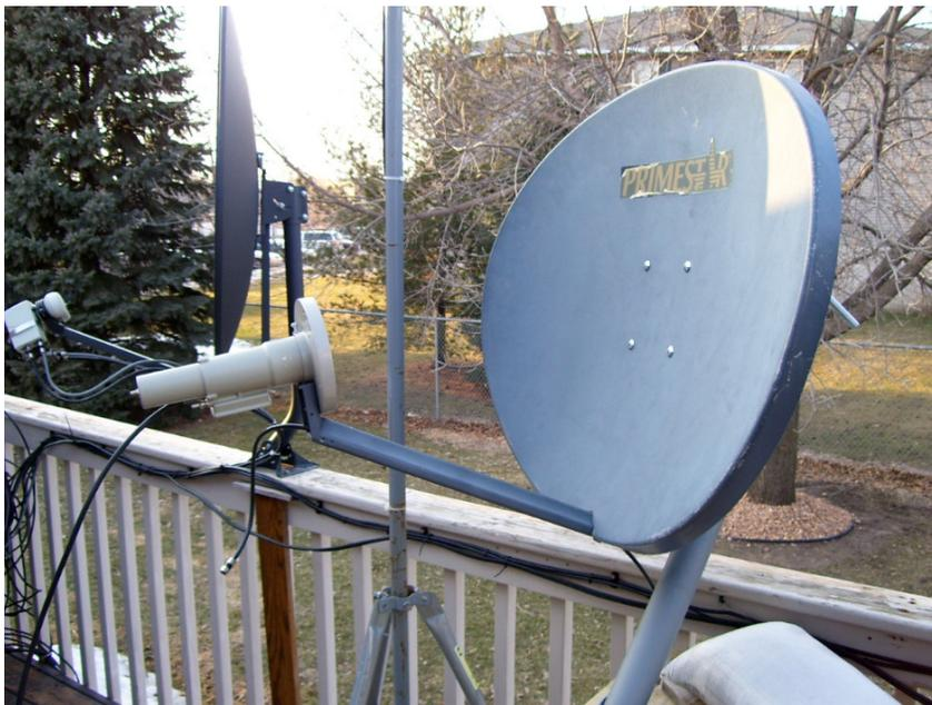
The picture above is the setup for C Band LNB. I have tried this on my 84e with mixed results. Only strong transponders can be viewed. At the time I am writing this I am working on seeing how the 1 meter will perform. It may do the same as this dish, I don't know. I have read that the 1.2 meter dish are really great with C Band. The bigger the dish, the more success on C Band.
