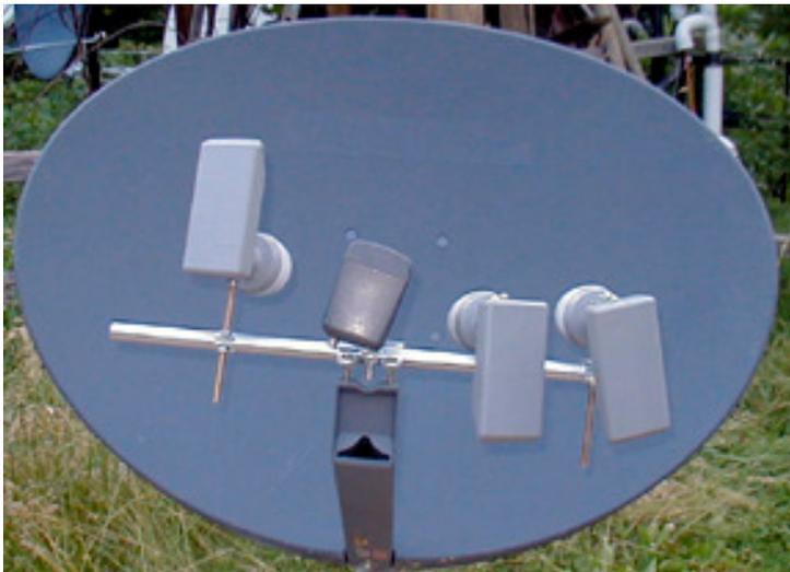
So as you can see, there are great potential on how to receive FTA signals using the Primestar dish and types of LNBF.
