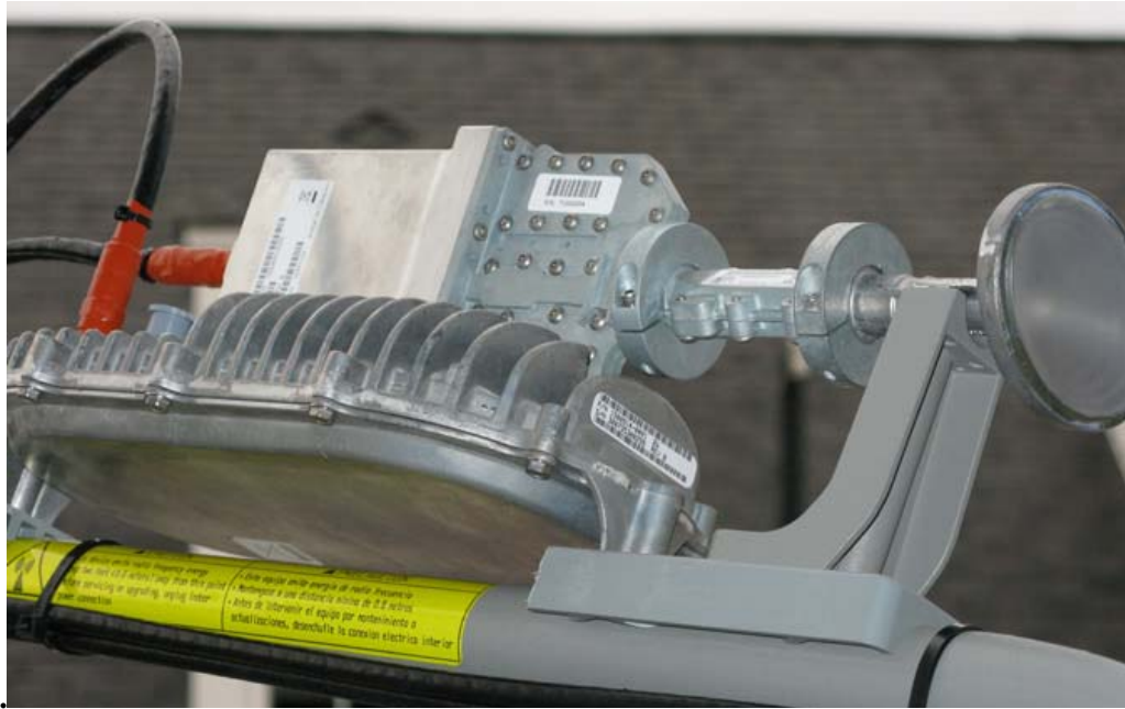
Figure 3. LHCP setting – Polarizer tilted to left when looking from the back of the radio
