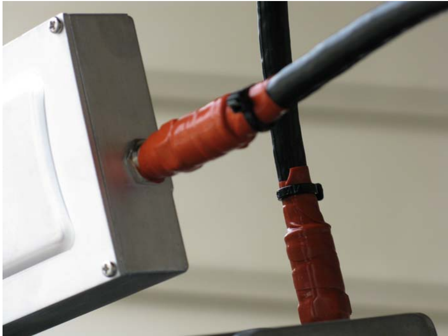
Figure 5. Weather proofing of connectors
