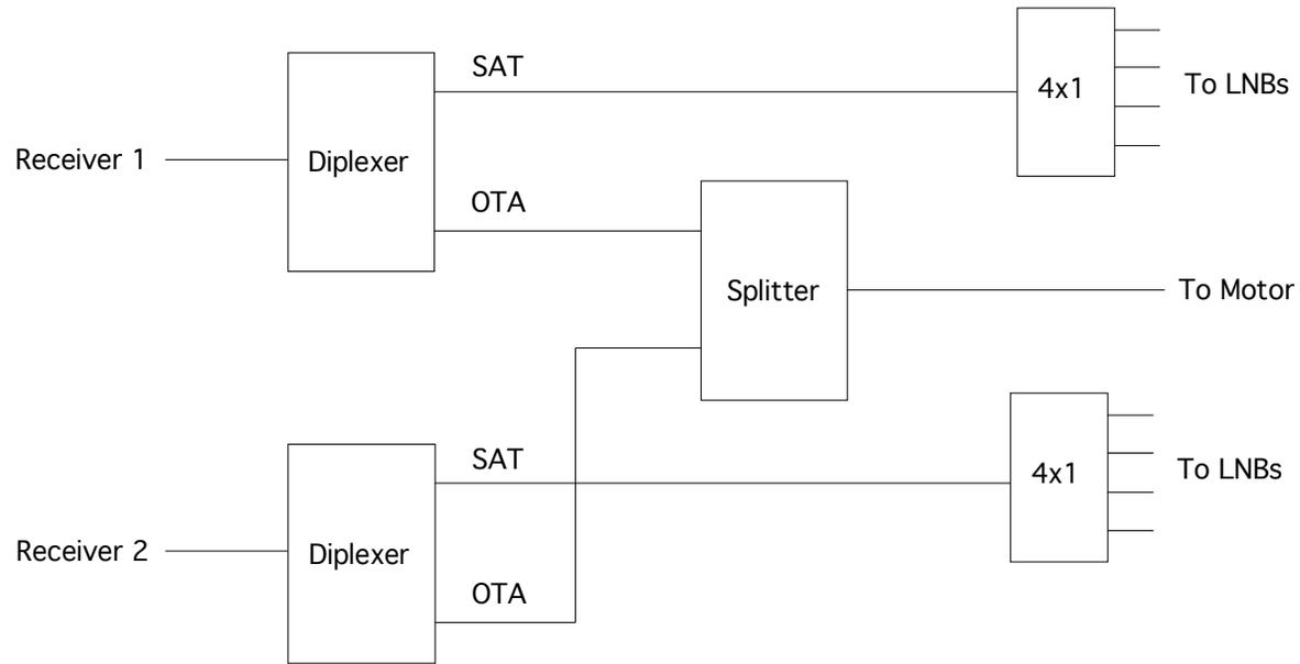
Note: both diplexers and the splitter must pass power on both ports!
