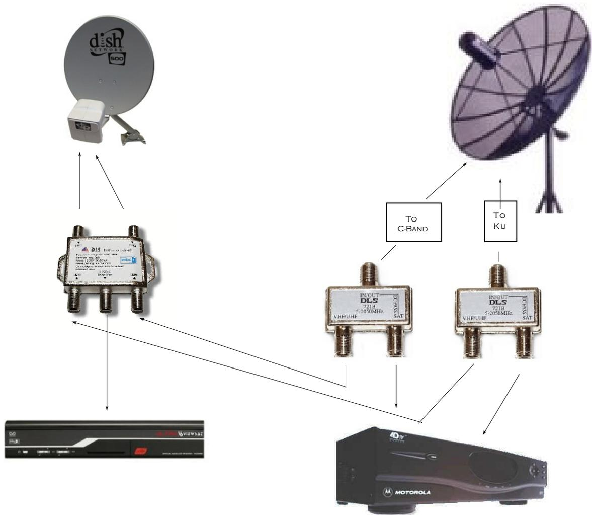
THIS SETUP INCORPORATED A FTA RECEIVER INTO YOUR EXISTING BUD C/KU BAND BUD SYSTEM.
