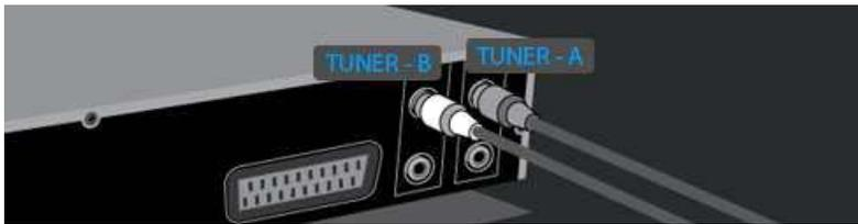
In this configuration both tuners are completely separated, meaning that you manually need to configure and scan for each tuner.
