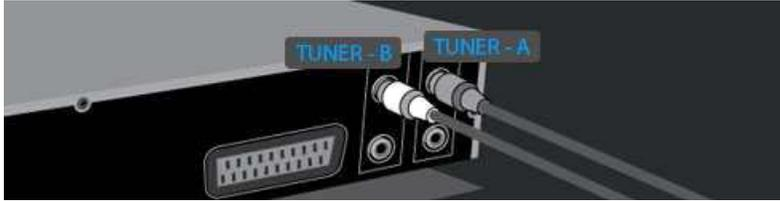
In this configuration you receive exactly the same satellites with the same antennas configuration but on 2 separated cables. For example you have a Monoblock LNB with multiple exits, or you have an external DiseqC switch with multiple exits. In this setup the Azbox automatically handles the switch from tuner-A to tuner-B when needed. For example you start recording a TV program you can zap and the Azbox will switch to tuner-B for you. It is transparent for you.
