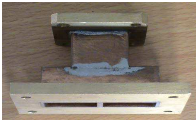
Figure 1: Photograph of a 1:2 power divider.
