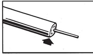
Cut the cable flush. Strip the outer jacket off 1/2", then trim the dielectric by cutting partially thru. **DO NOT NICK THE CENTER CONDUCTOR!** Twist and pull off leaving a 1/2" minimum of exposed center conductor.
