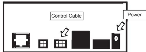
Attach the TRAV'LER control cable to the TRAV'LER Interface Box, as shown in Figure 5A. Attach the output cable from the Power supply to the TRAV'LER Interface Box. See above. Finally, connect a coax cable from the TRAV'LER mount to each of the receivers being used with the TRAV'LER Automatic Satellite Dish. See Appendix for information on properly installing a Hex Connector.
