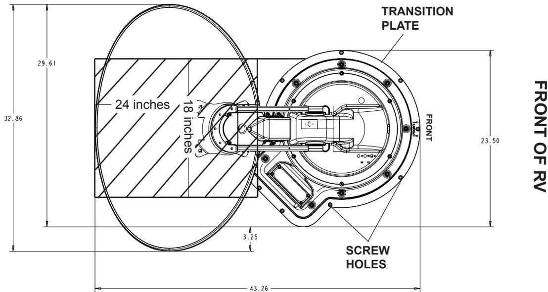
**NOTE: Anything in the striped area will interfere with the operation of the TRAV'LER antenna and may cause damage to the object or the TRAV'LER antenna.**
