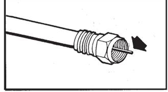
**IN COLD WEATHER OR INDOORS:** Trim off center conductor leaving it extended 1/16" of an inch beyond the connector. (Use diagonal pliers for cutting center conductor).
