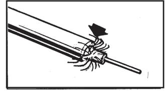
Remove additional 1/4" of the outer jacket. Pull the braid away from the dielectric and fold over the jacket. If there's any residue on the center conductor scrape off with non-metallic object.
