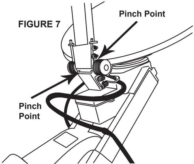
Using the (4) bolts and nuts provided, attach the reflector to the mounting bracket.
