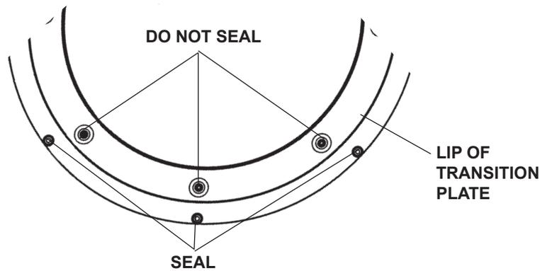
Run a solid bead of sealant around the transition plate, making sure to cover each screw head. Be careful not to get any sealant above the lip of the transition plate. See diagram of transition plate.
