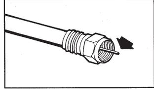
**IN HOT WEATHER:** Trim off center conductor leaving 3/16" beyond the connector. The center conductor expands at higher temperatures. If a little extra is not provided, it may contract enough in the winter to create an open connection and result in loss of picture.
