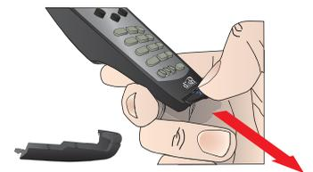
**B** Flip the key and re-insert it into the remote so that the green TV1 side of the key is facing up.
