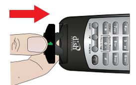
**C** Use the tip of a pen to slide the switch located in the remote battery compartment to the IR position. Replace the battery cover.
