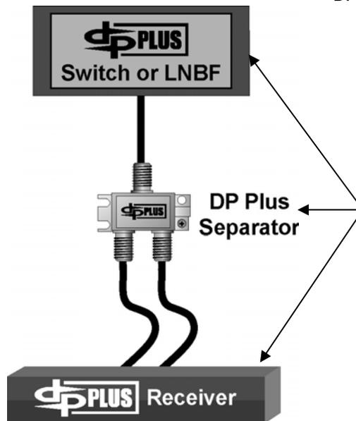
**For the single-cable dual-tuner advantage, all three components must be DISH Pro Plus.**
