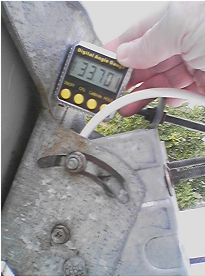
The dish elevation is set to 61 degrees and subtracting the 33.7 degrees read on the dish bracket results in the offset of 27.3. That meets the published specification for the dish.
