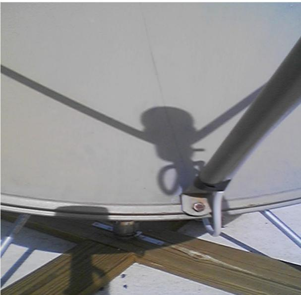
At Solar Noon rotate the azimuth of the dish until the shadow of the LNBF falls on the centerline of the dish.
