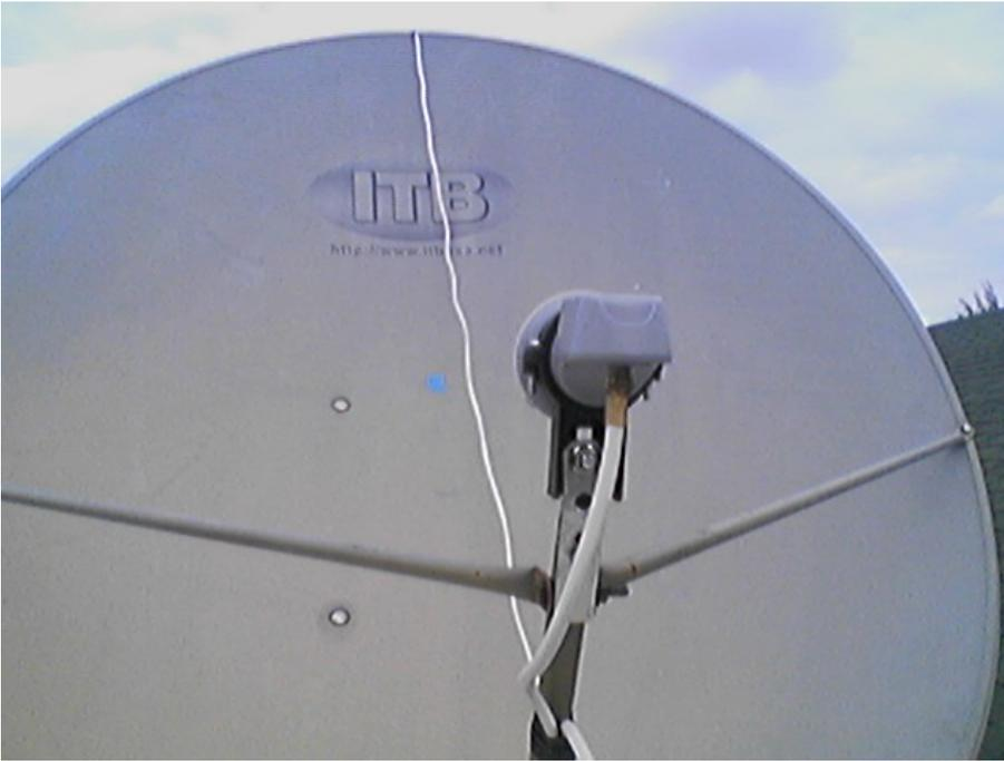
Use the string and adjust the LNB so that the lens face just touches the string at “c”. Note the blue tape on the dish, this was determined to be the focal center of the dish. The focal length of 35” for this dish made it necessary to aim the LNB upward and not at the apparent center of the dish.
