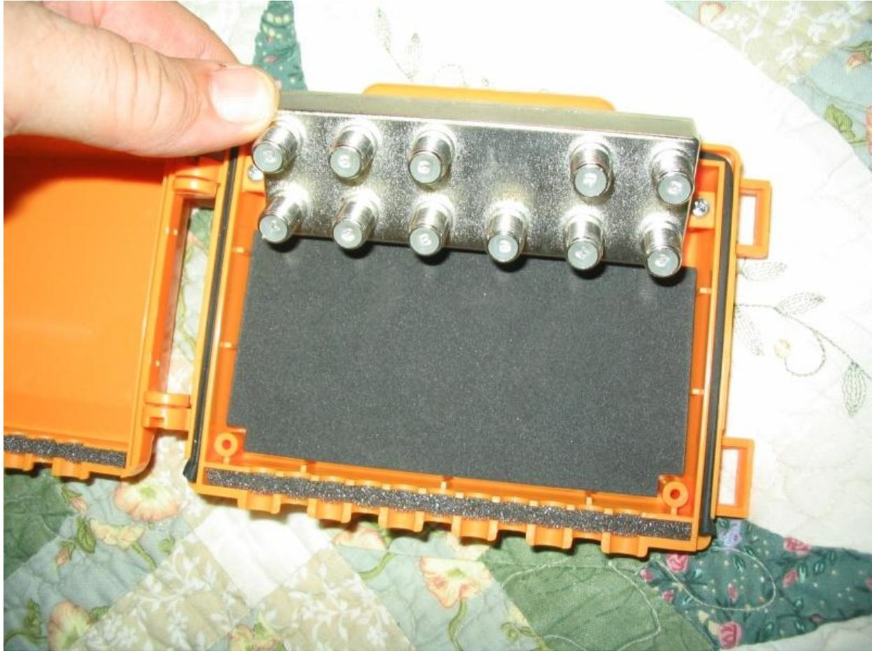
The switch is labeled as “programmable”. Since I had no prior background on this type of DiSEqC switch I had to do a bit of searching on the internet to discover some of the details. The switch can be programmed by the user to conform to whatever mode is needed for the situation, and has 8 different modes available...
